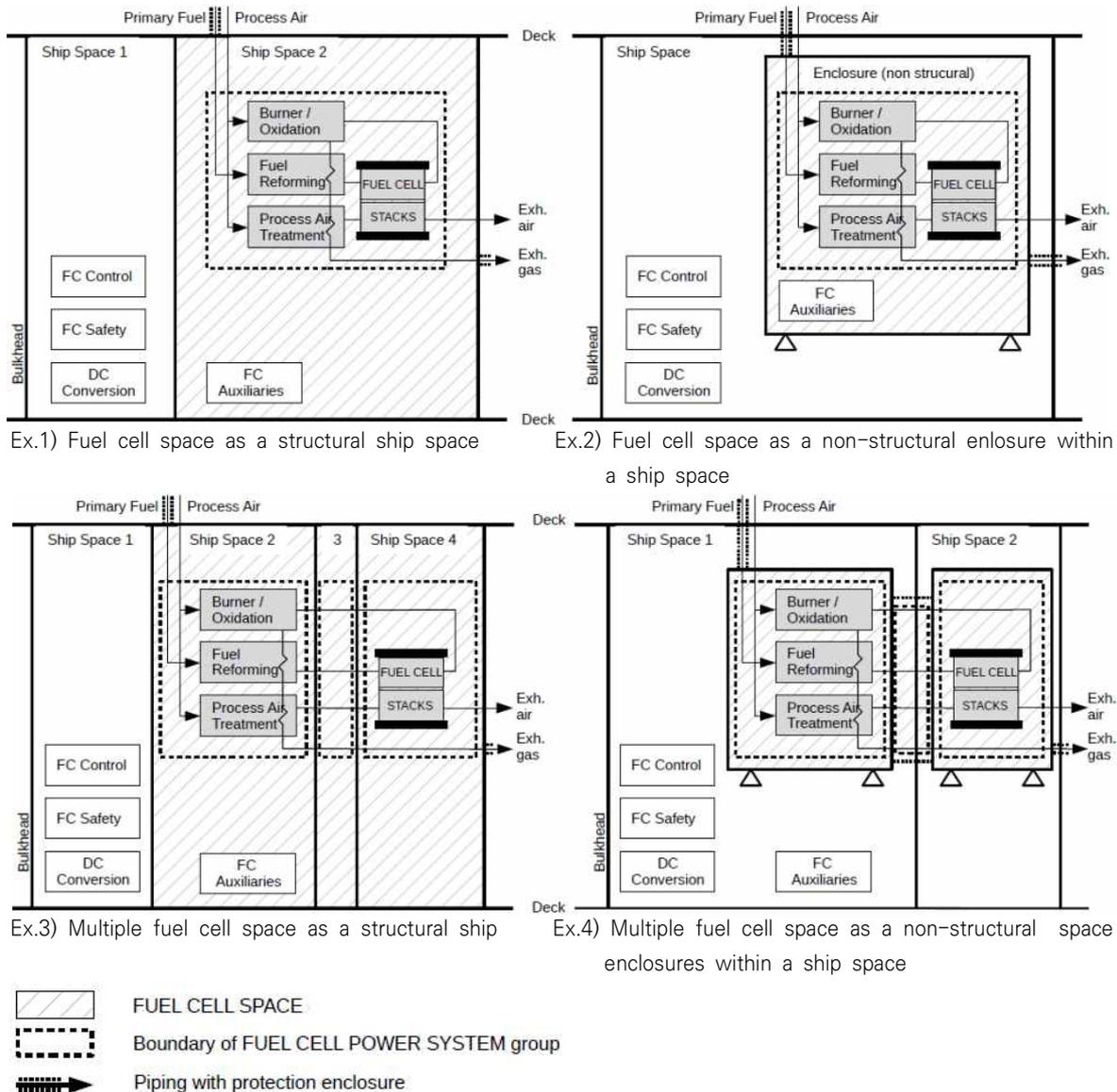
Fig 1.2 Examples for Fuel Cell Spaces
