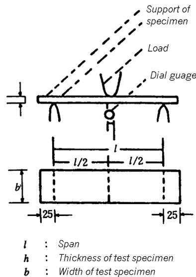
Fig 3.2 Bending Strength Specimens of Structural Plywood
