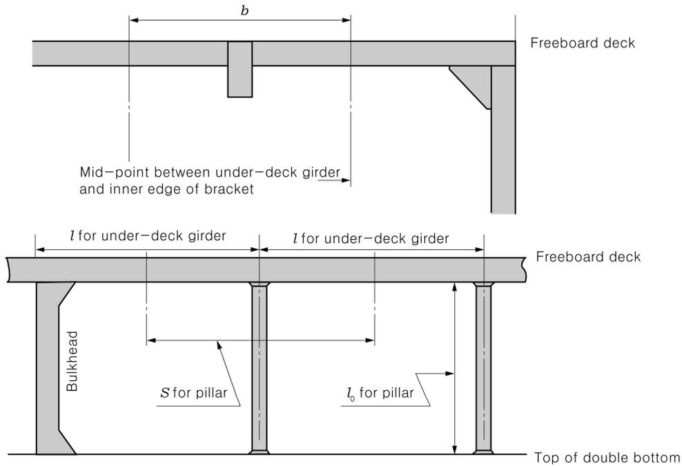
Fig 11.1 Measurement of  $b$ ,  $l$ ,  $S$ , and  $l_0$
