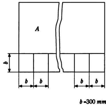
Fig 1.3 Selection of Test Specimens from Fibreglass Reinforcements
