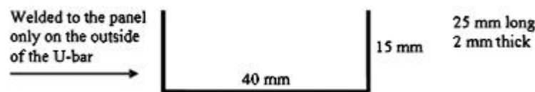
Fig 3.30.1 Welding of U-bar
